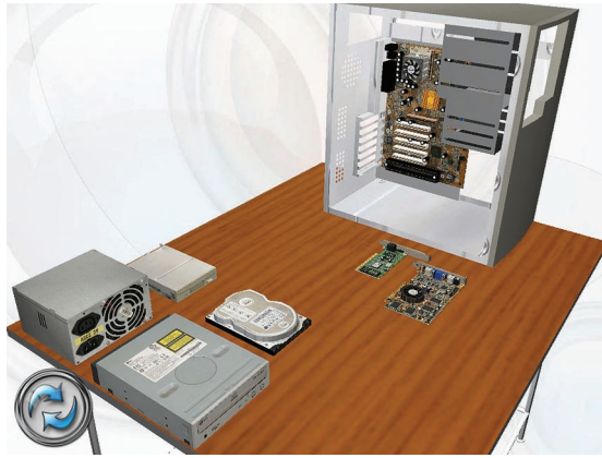
Figure 3. Building a PC. After installing the main components into the PC case — in the right sequence — the user can go inside the case, take a walk around, and see how it all fits together.
