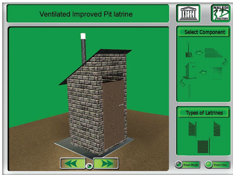
Figure 4. How to build a VIP(ventilated, improved pit) latrine. In this simulation, the VIP latrine is built step by step and explains the importance of the ventilation pipe facing the equator. This is the most important design feature that has led to several “ahha” moments with audiences.
