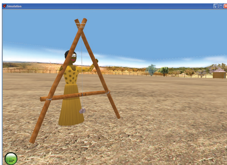
Figure 7. Surveying fields to conserve soil. It's important to plough along the contour line to minimize water run-off, which can carry away lots of soil.
